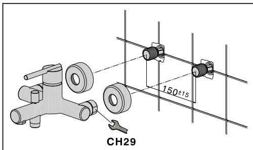
**SOSTITUZIONE DELLA VALVOLA MISCELATRICE A DISCHI CERAMICI**
