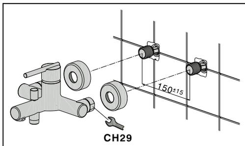
**SOSTITUZIONE DELLA VALVOLA MISCELATRICE A DISCHI CERAMICI**
